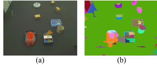
Fig. 3. Segmentation Result—(a) Original image. (b) Segmented image.
